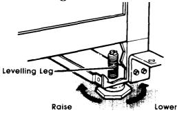
This refrigerator has 2 threaded levelling legs that are shipped in a separate package.
